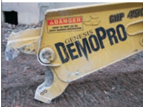
Pac Man's jaw: the Genesis Demo Pro attachment is capable of taking bites out of concrete and steel
